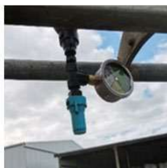
Bottom entry ¼" Isometric 63 mm Gauge fitted on a ¼" Tee with Quick TeeJet cap*
