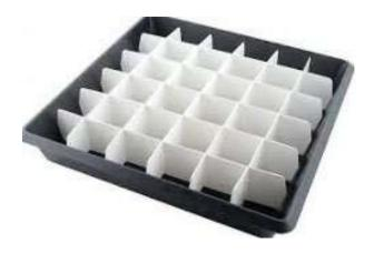
b. Collectors should collect a reasonable amount of the swath. For most spreaders it has been found that about 20 trays at a one-metre interval provides sufficient information to allow sound assessments of spreader performance to be made.
